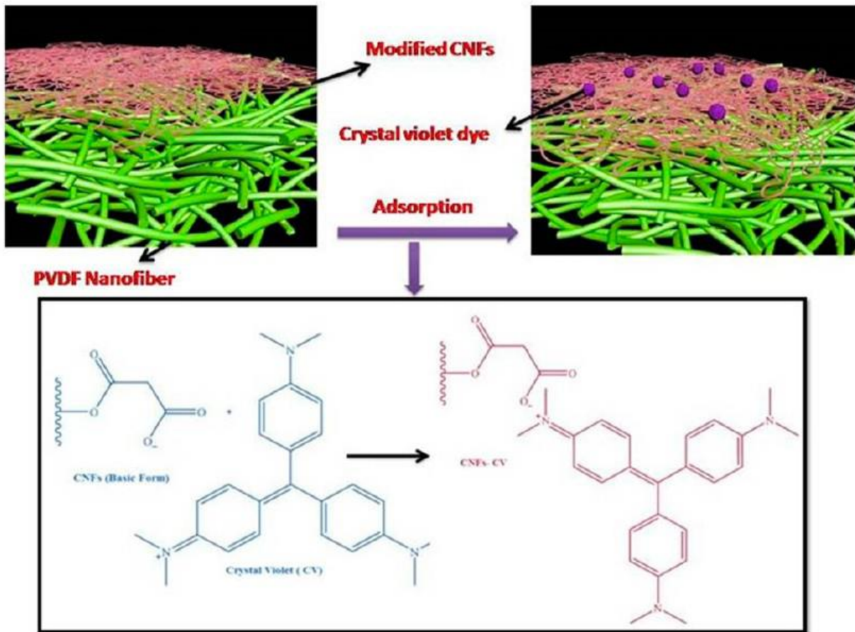
Schematic Representation of crystal violet dye removal by Meldrum's acid- modified CNF-based PVDF nanofibrous membrane and its mechanism.
